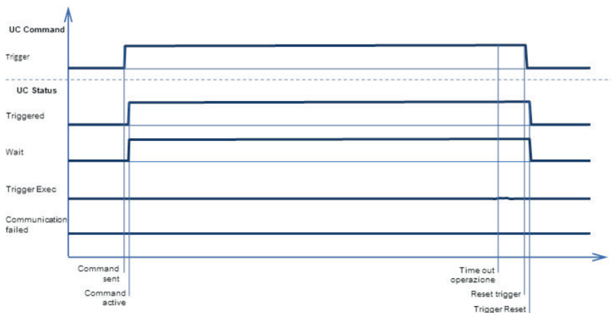
Fig. 10 5 – Timing flag in case of unreachable device
